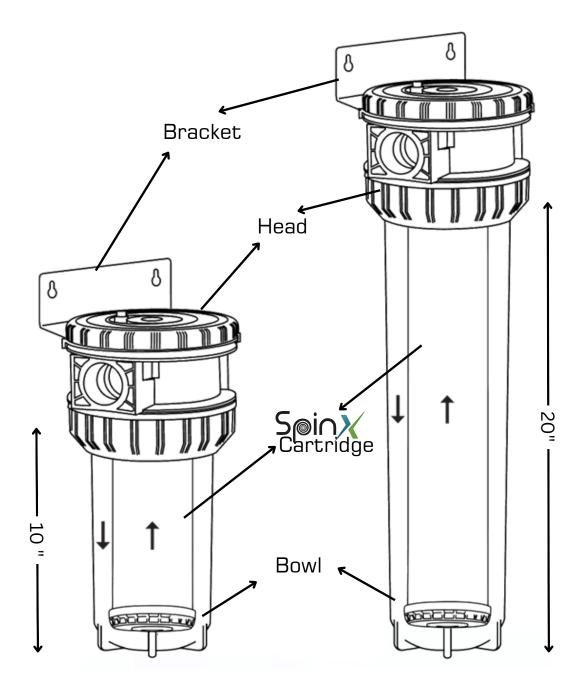
Watch Water's ScaleTech cartridge systems provide protection scale on internal and external plumbing surfaces. Our cartridge-based systems can be installed on a coldwater line before a waterusing device (water heater, hot-beverage system, appliance, steamer, etc.) needs that hard water protection.
