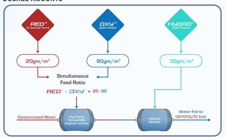
Please note: The values provided here in this diagram are just reference values. The actually dosing amount will vary on site and will in fact be much lower than the values given here. The exact dosing amount should be estimated beforehand by the customer using our Lab Test-kit.
