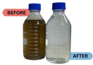
The complex and persistent organic chemicals found in petrochemical effluent make typical treatment procedures ineffective. To address these problems, Watch Water, after thorough research developed a five-stage purification process including Catalyst, Coagulation, Oxidation, Adsorption and finally Polishing. The whole process is called **REDOXY VAOP**.
