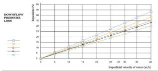
Bed Expansion and Pressure Loss curves are provided for the most commonly used particle size.
