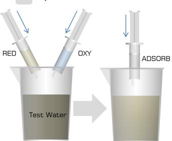
Put 1 liter of test water in the plastic mug and inject RED & OXY simultaneously with both hands. Stir the mixture for 1 minute. Add ADSORB to the mixture and stir for 1 minute. Leave the solution in rest for 10 minutes.
