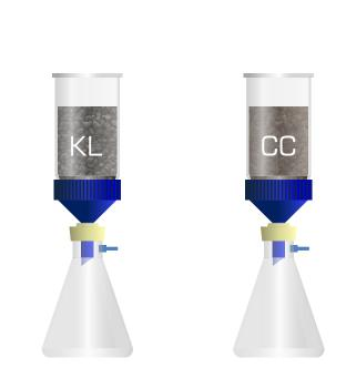
2. Put Katalox-Light and Catalytic Carbon from the respective 1 liter bag and pour the media in two filter set up
