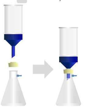
Assemble The Filter head to fit on the Filter Flask with the help of the Adapter. Prepare two sets one for Katalox-Light and one for Catalytic Carbon.
