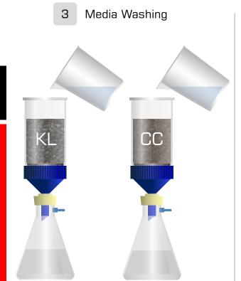
3. Pour one liter of clean water (with the mug) through both KL and CC media. Fines might be observed. Throw away the water collected in the filter flasks.
