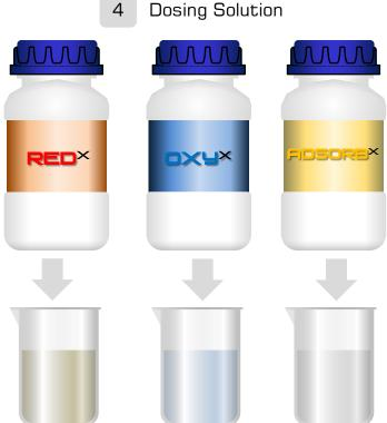
Prepare the dosing solution from the respective chemical diluting them in the water. Dilution strength is contaminants dependent. See **RED-OXY Part I** for more information.
