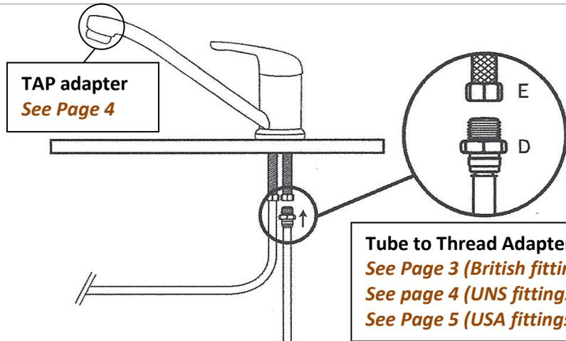
**Tube to Tube/Thread Adapter**
