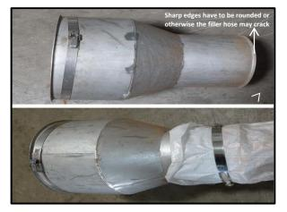
During the filling process, the hose should be lifted consistently, so that it always remains above the surface of the material and does not get jammed in the material. This is even more important for large drop heights!
