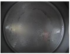
Mineral left over after boiling 20 L of SPECIAL Filter (Model : SP 520) Treated Water Image Source: Brita® (Feb., 2014)
