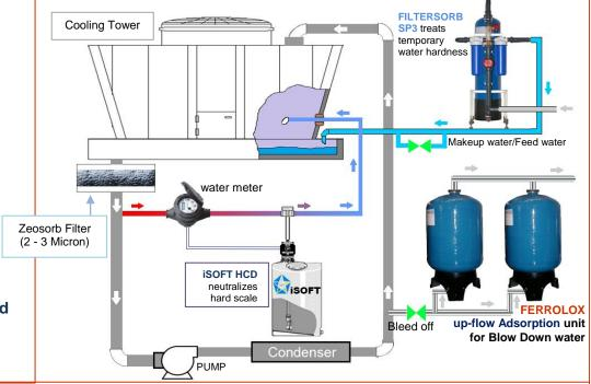
Typical Cooling loop with complete Scale Prevention + Corrosion Control + Blow Down Solution
