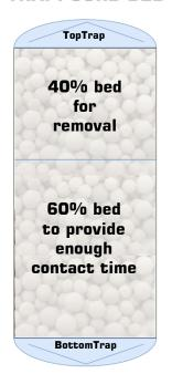
TRAPPSORB systems are normally designed as packed bed system, where 40 % of its bed can be considered for the consumption during the treatment and 60% bed should always be there to provide enough contact time for the treatment.
